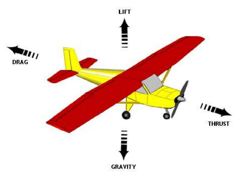
So for airplanes to fly, the thrust must be greater than the drag and the lift must be greater than the gravity (so as you can see, drag opposes thrust and lift opposes gravity).
