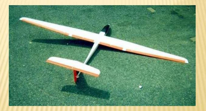
If we are breaking the wing in two parts then we have an advantage that we can give dihedral angle to the wing.
